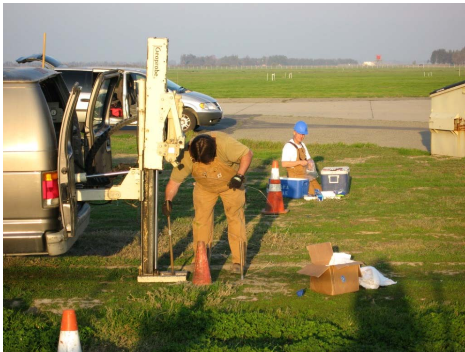
Photograph 9: EPA installing micro-purge soil gas probes.
