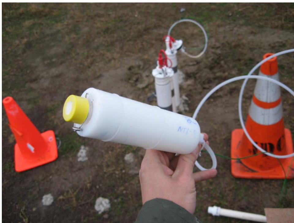
Photograph 15: PDS vial (with yellow cap) in holding device.
