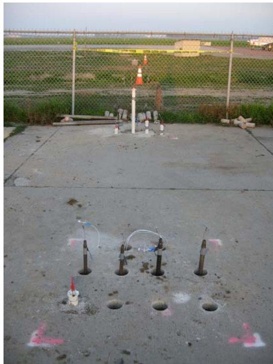
Photograph 12: Southern transect looking east. Micro-purge probes in foreground, macro-purge probes and sub-slab probe behind micro-purge probes.
