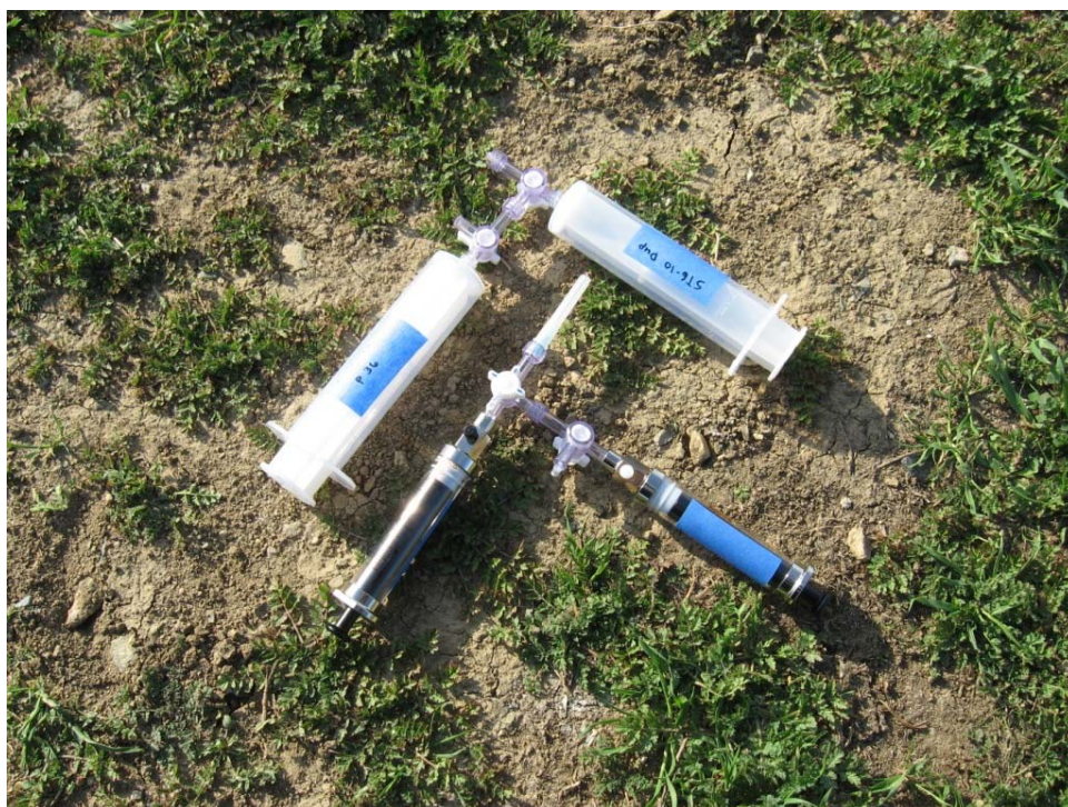
Photograph 16: Polypropylene (upper) and glass (lower) sampling syringes.
