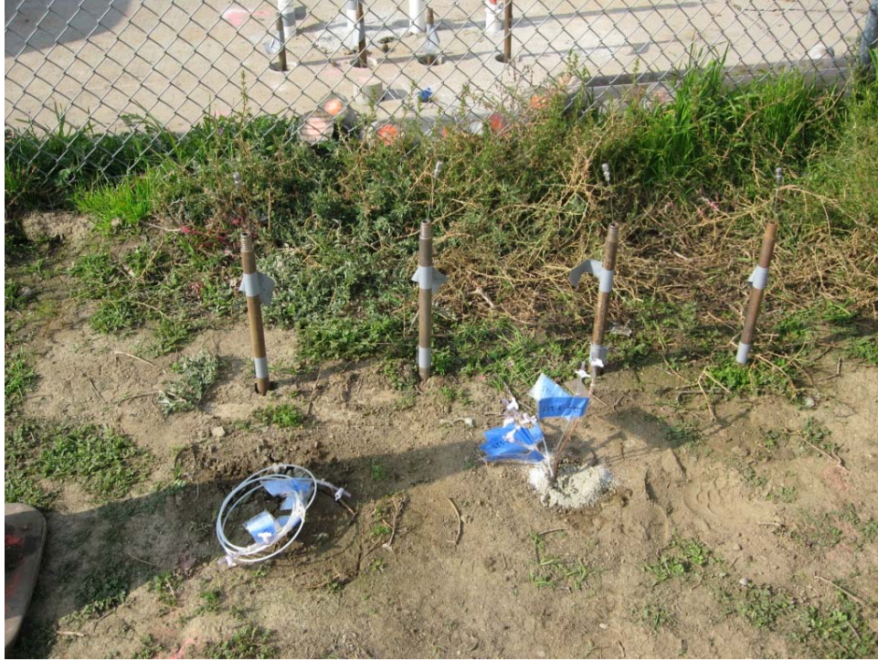
Photograph 13: PDS wells in background, micro-purge probes in middle ground, macro-purge probes and tubing-type cluster in foreground.
