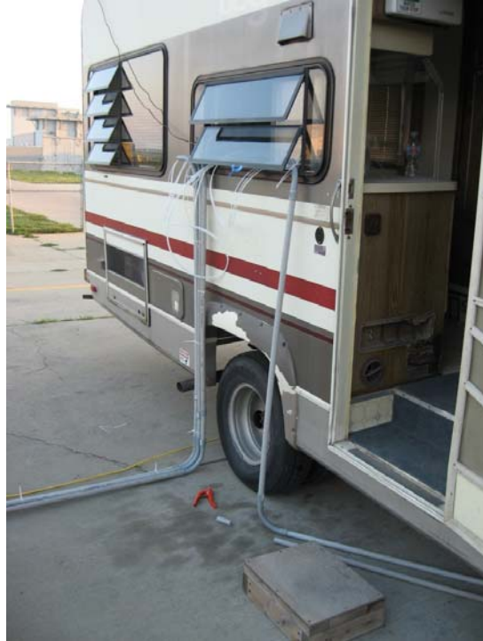
Photograph 17: Auto-sampler RV. Conduit containing Nylaflow tubing from macro-purge probes on left.
